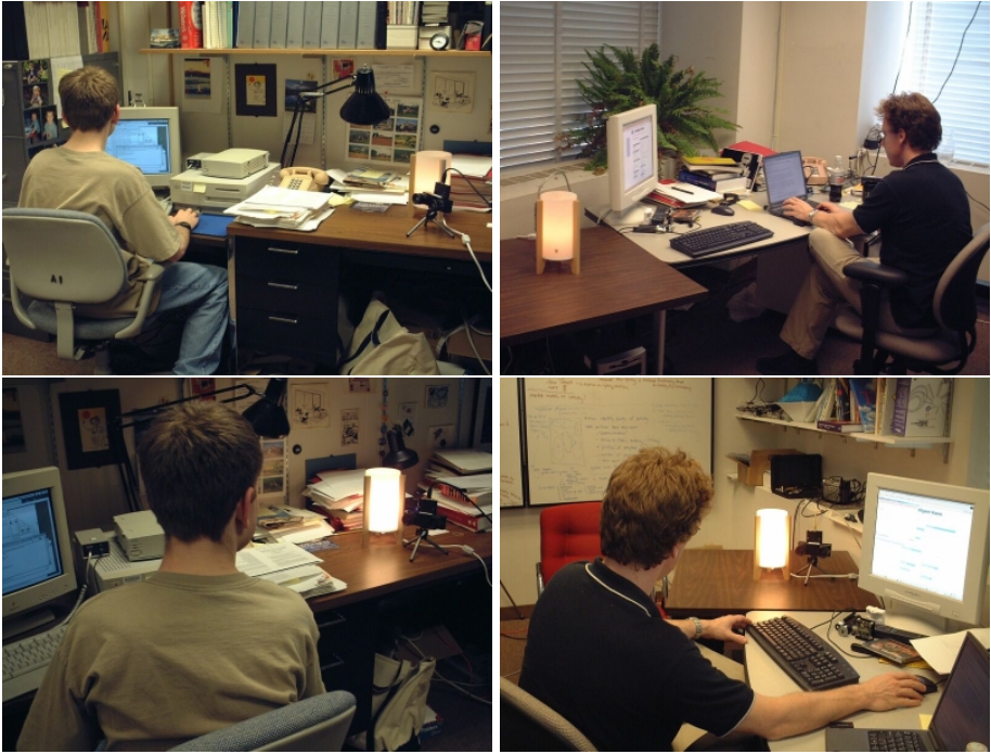
Fig. 5. The two upper images show the level of physical presence when both users are in their office but not explicitly looking at the lamp (which is dim). In the lower images, one of the users has noticed his lamp getting brighter and has returned that gaze.
